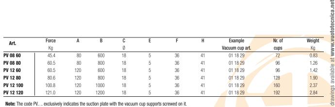
Note: The code PV.... exclusively indicates the suction plate with the vacuum cup supports screwed on it.
